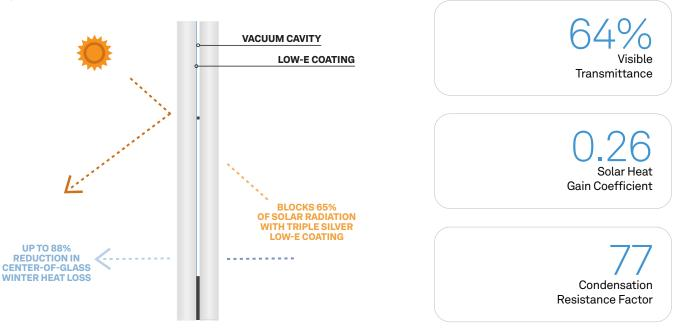
1. Comparing to Double Pane Clear for Glass-Only Retrofit • 2. Center of Glass U-Value comparison of Enthermal Triple Silver on surface 2 (U-Value 0.056) vs. Double Pane IG, Air Fill (U-Value 0.473).
